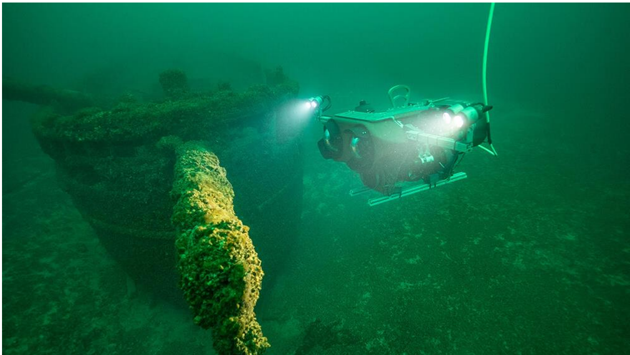
Figure 3.7. Pixel , a remotely operated vehicle, shines its lights on a shipwreck. Photo: Marine Imaging Technologies/NOAA
